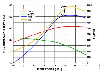
Figure 31. Output Power (Pout), Gain, Power Added Efficiency (PAE), and Supply Current (IDD) vs. Input Power at 3.8 GHz
