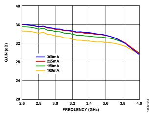
Figure 13. Gain vs. Frequency at Various Supply Currents
