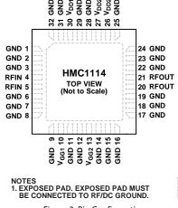
Figure 2. Pin Configuration
