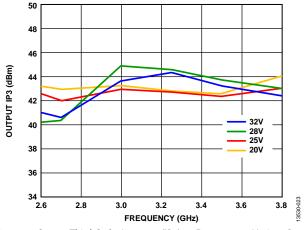
Figure 23. Output Third-Order Intercept (IP3) vs. Frequency at Various Supply Voltages, P<sub>OUT</sub>/Tone = 30 dBm
