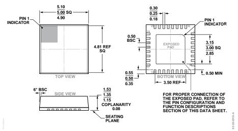
Figure 43. 32-Lead Lead Frame Chip Scale Package, Premolded Cavity [LFCSP\_CAV]
