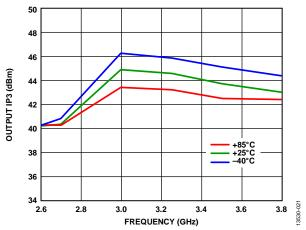
Figure 21. Output Third-Order Intercept (IP3) vs. Frequency at Various
