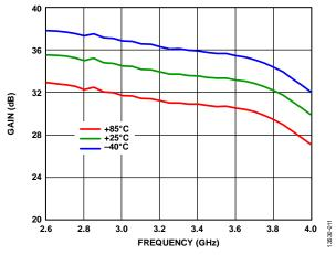
Figure 11. Gain vs. Frequency at Various Temperatures
