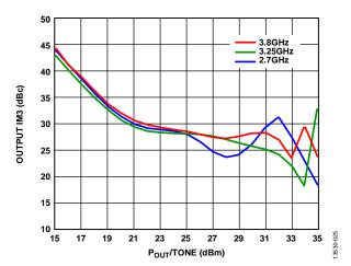
Figure 25. Output Third-Order Intermodulation (IM3) vs.  $P_{OUT}/Tone$  at  $V_{DD} = 20 \text{ V}$
