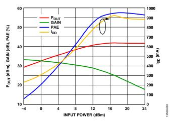
Figure 30. Output Power (Pout), Gain, Power Added Efficiency (PAE), and Supply Current (IDD) vs. Input Power at 3.2 GHz
