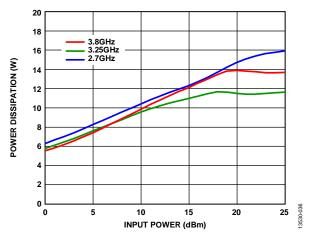
Figure 36. Power Dissipation vs. Input Power at 85°C
