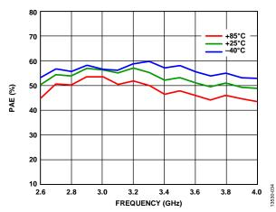
Figure 34. Power Added Efficiency (PAE) vs. Frequency at Various Temperatures,  $P_{\rm IN} = 16~{\rm dBm}$
