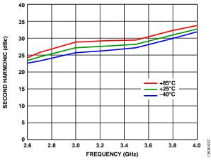
Figure 37. Second Harmonic vs. Frequency at Various Temperatures,  $P_{OUT} = 30 \text{ dBm}$
