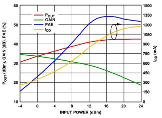
Figure 28. Output Power ( $P_{OUT}$ ), Gain, Power Added Efficiency (PAE), and Supply Current ( $I_{DD}$ ) vs. Input Power at 2.7 GHz
