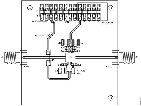
Figure 42. Evaluation Printed Circuit Board (PCB)
