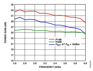
Figure 22. Power Gain vs. Frequency
