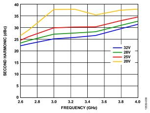
Figure 38. Second Harmonic vs. Frequency at Various Supply Voltages,  $P_{\text{OUT}}$  = 30 dBm
